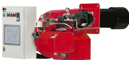
Burners for diesel two stages progressive (hi-low flame) or modulating (PID fully modulating) with the addition of the optional system modulation kit plus feeder. Fan at high pressurisation, combustion head with adjustment at high efficiency and high flame stability.
