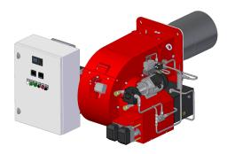
Burners for heavy oil at three stages, fan at high pressurisation, combustion head with adjustment at high efficiency and high flame stability complete of servomotors for the opening of the air shutters, suitable for heavy oil up to  $20^{\circ}\text{E}$  to  $50^{\circ}\text{C}$  and for BTZ heavy oil.
