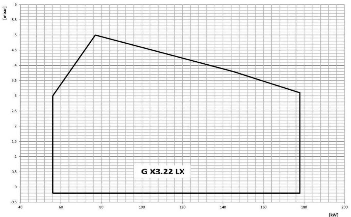
Fig. 4 X = Thermal power Y = Pression in the combustion chamber
