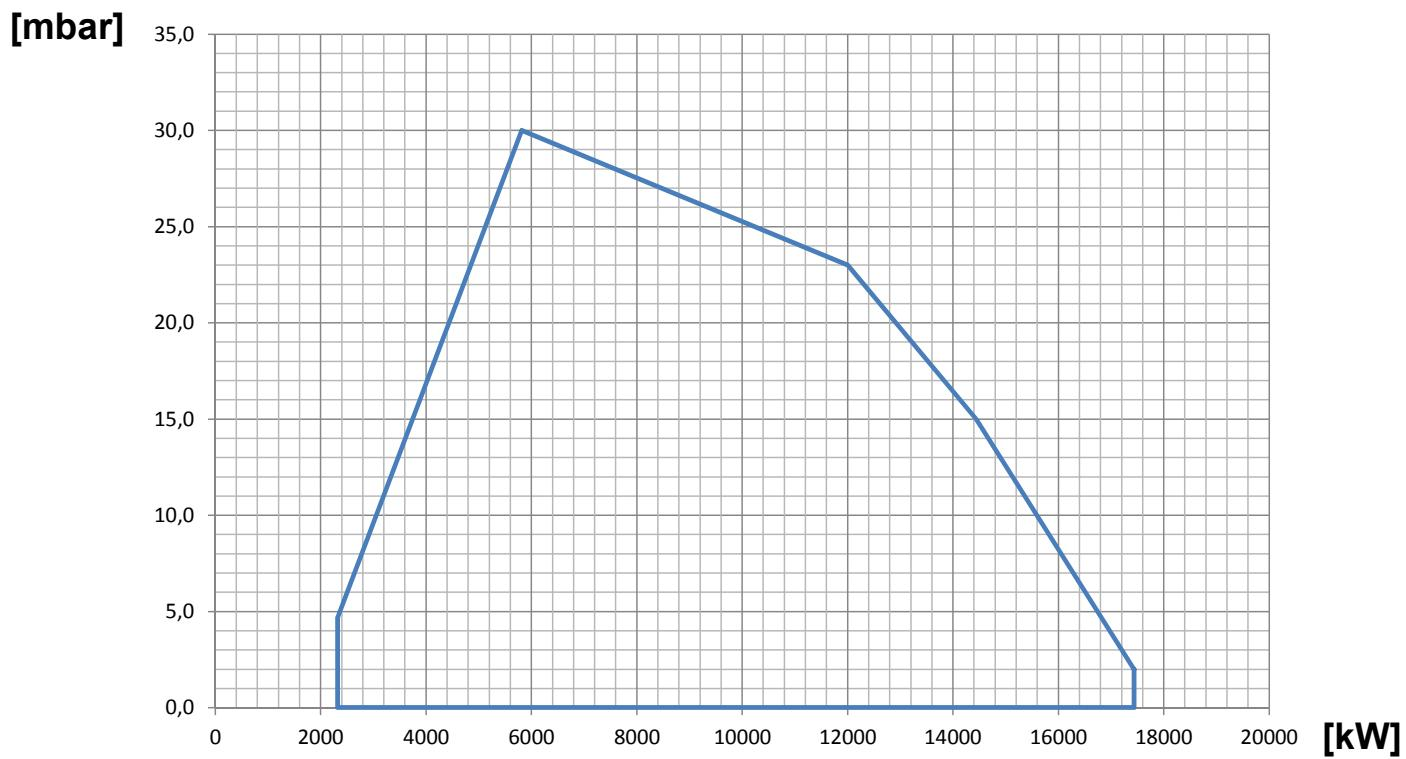
**Fig. 7** X = Thermal power Y = Pressure in the combustion chamber
