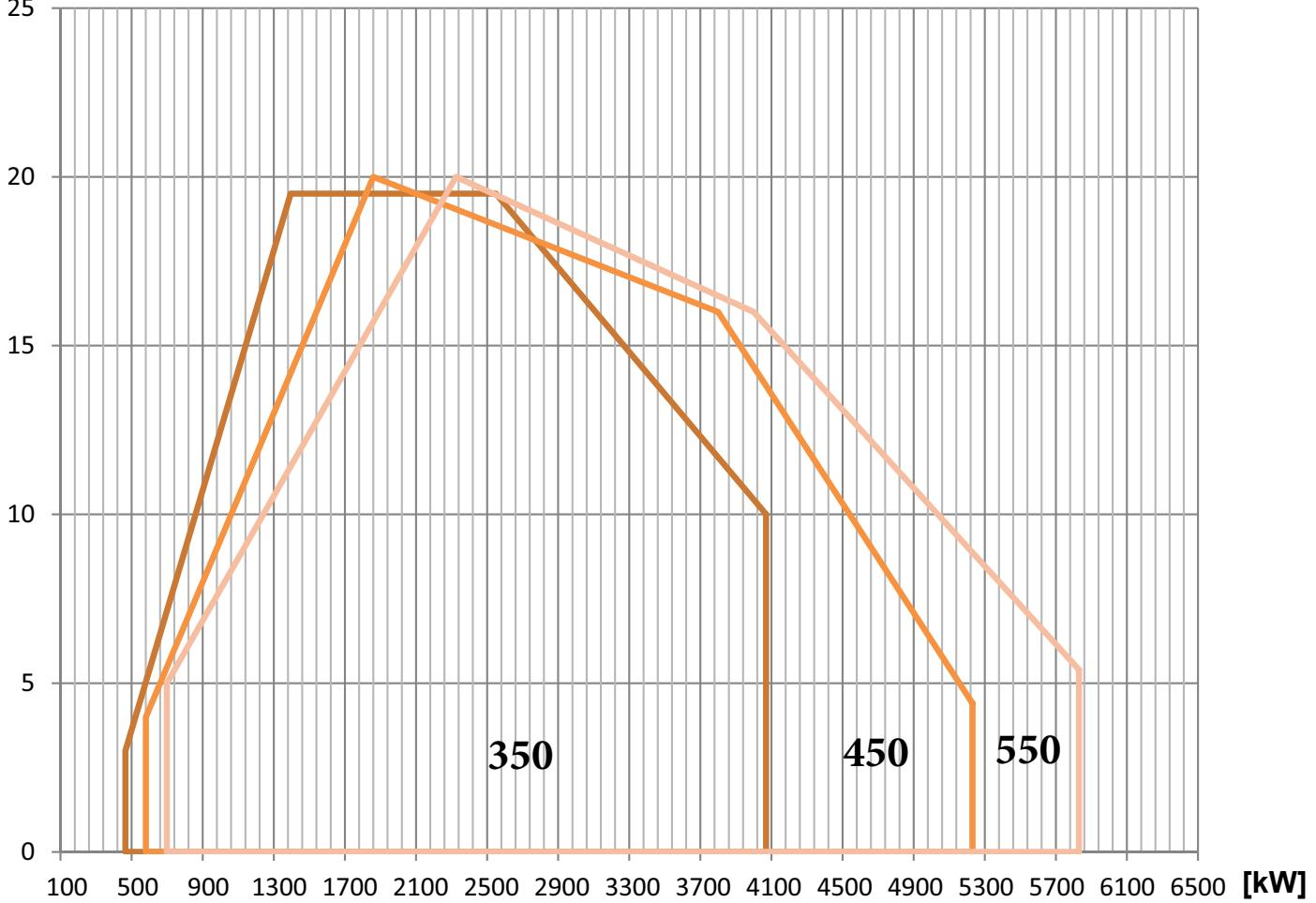
**Fig. 5** X = Thermal power Y = Pressure in the combustion chamber
