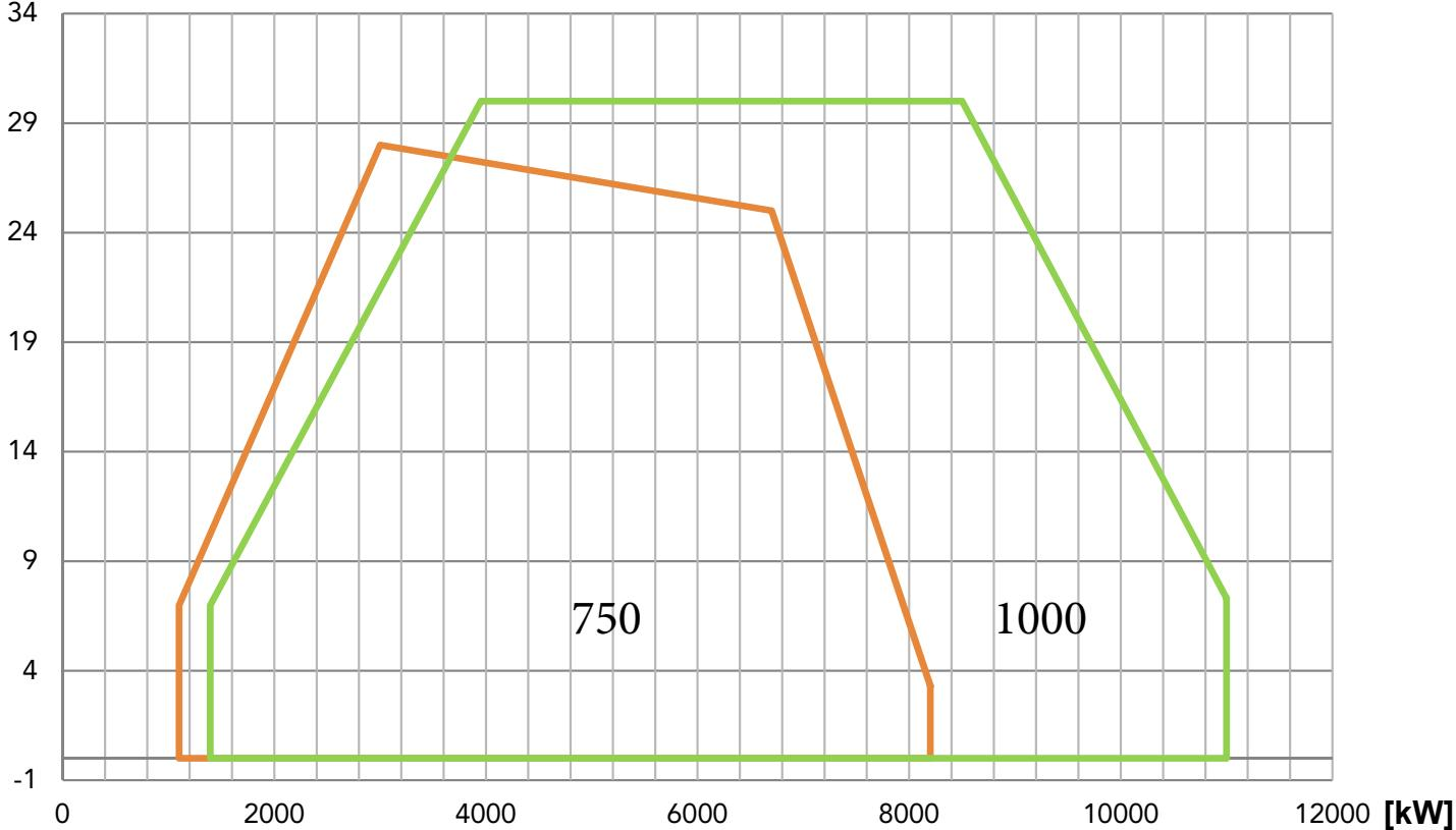
**Fig. 6** X = Thermal power Y = Pressure in the combustion chamber
