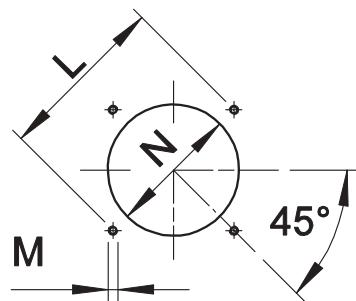
\* Suggested dimension of connection between burner and generator.
