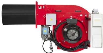
Burners for gas two stages progressive (hi-low flame) or modulating (PID fully modulating) equipped with electronic control box (Lamtec BT3). Fan at high pressurisation, combustion head with adjustment at high efficiency and high flame stability. Equipped with ignition pilot flame.
