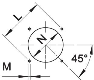
The dimensions of the boiler plate must be as indicated in the drawing.
