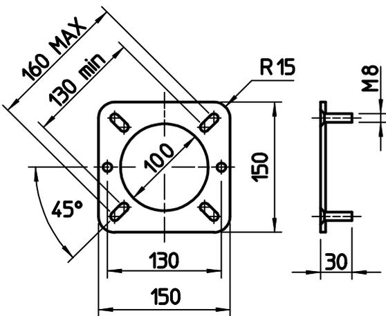
**Fig. 4** Boiler plate
