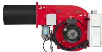
Burners for gas two stages progressive (hi-low flame) or modulating (PID fully modulating) equipped with electronic camme (Lamtec Etamatic). Fan at high pressurisation, combustion head with adjustment at high efficiency and high flame stability. Equipped with ignition pilot flame.
