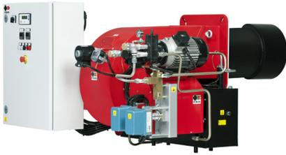
Burners for heavy oil two stages progressive or PID fully modulating with the addition of the optional system modulation kit plus feeder. Fan at high pressurisation, combustion head with adjustment at high efficiency and high flame stability complete of servomotor for the opening of the air shutters, suitable for heavy oil up to 20°E to 50°C and for BTZ heavy oil.
