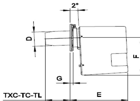
\* Suggested dimension of connection between burner and generator
