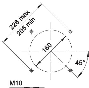
The dimensions of the boiler plate must be as indicated in the drawing.
