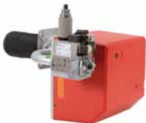
Burners for gas, double stage, aluminium frame, protection cover with noise reduction plate, combustion head with adjustment at high efficiency and high flame stability.
